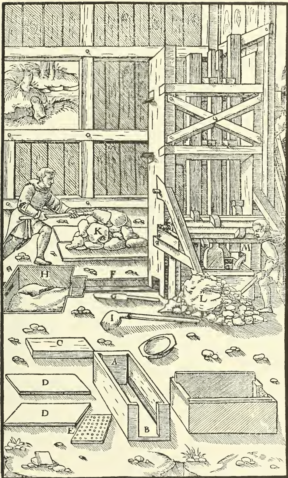
A—MORTAR. B—OPEN END OF MORTAR. C—SLAB OF ROCK. D—IRON SOLE PLATES. E—SCREEN. F—LAUNDER. G—WOODEN SHOVEL. H—SETTLING PIT. I—IRON SHOVEL. K—HEAP OF MATERIAL WHICH HAS SETTLED. L—ORE WHICH REQUIRES CRUSHING. M—SMALL LAUNDER.
